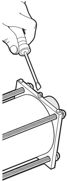
*Adjustments can be made to the launcher in order to accommodate rocket cars of varying sizes*
